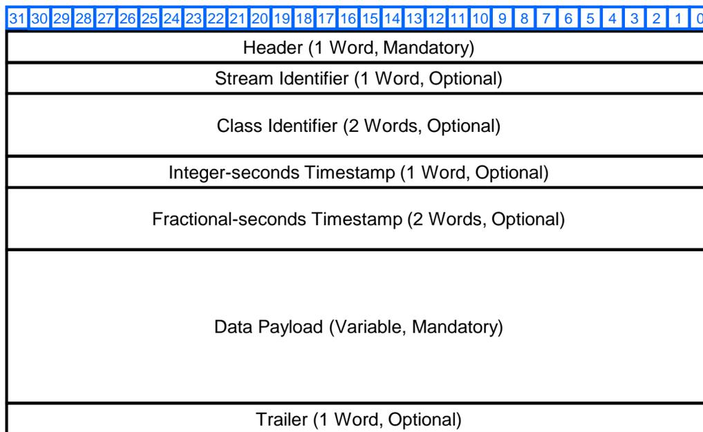
**Figure 3-1 VRT (VITA 49.0) IF Data Packet Format**
