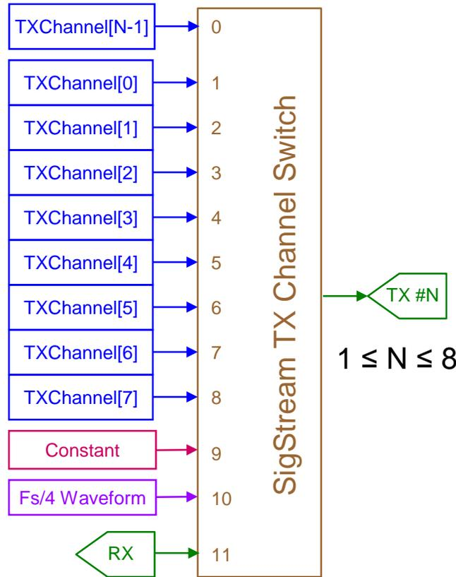
**Figure 5-2 TX Switch Select Settings**
