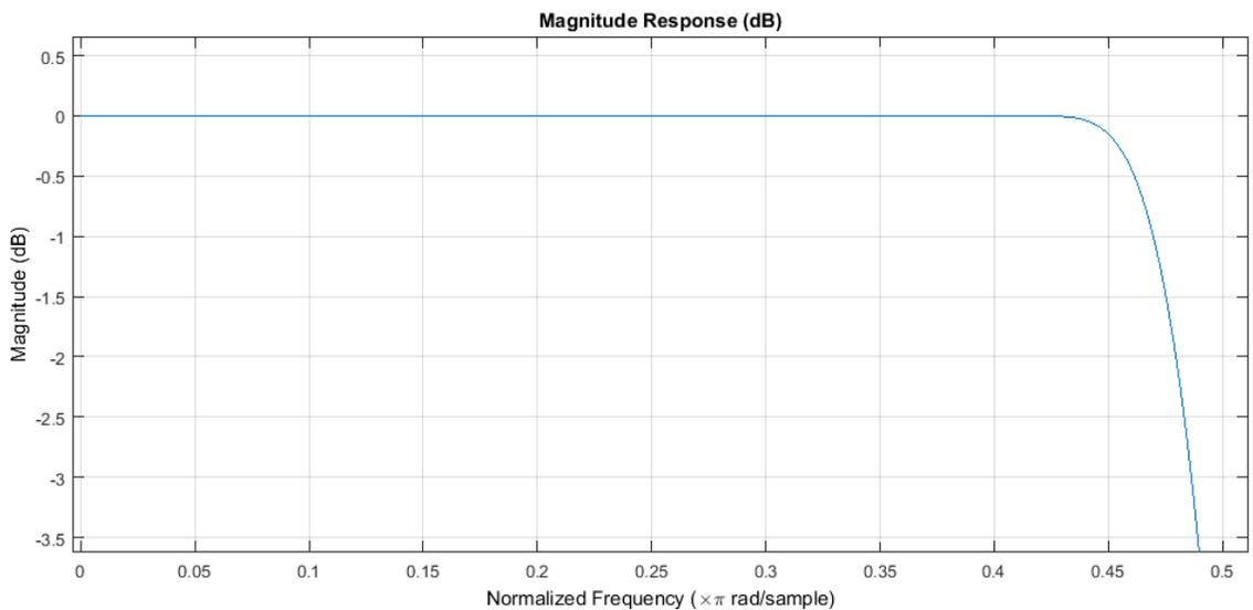
**Figure 2-6 Halfband Filter Passband**
