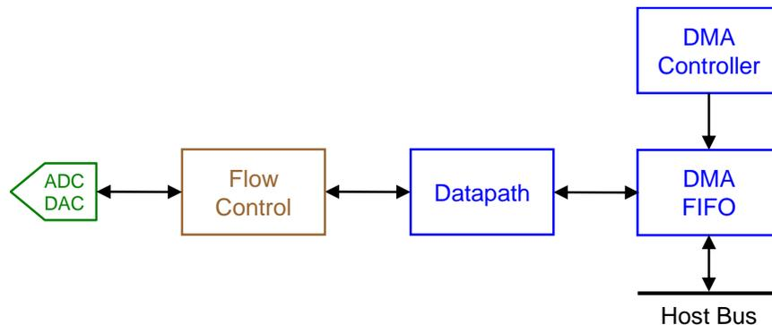
Figure 5-3 TX/RX Data Flow
