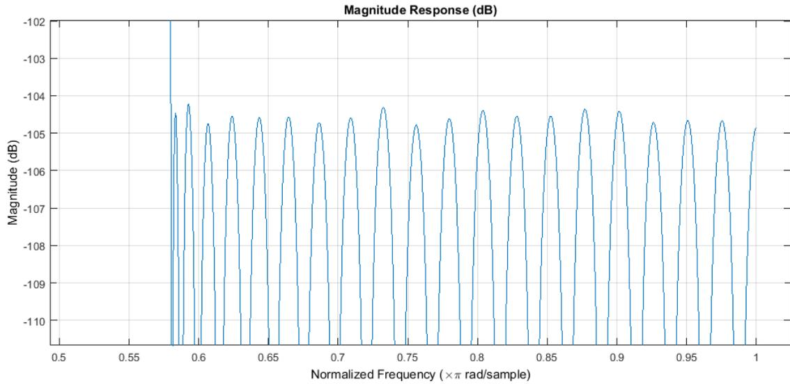
**Figure 2-5 Halfband Filter Stopband**
