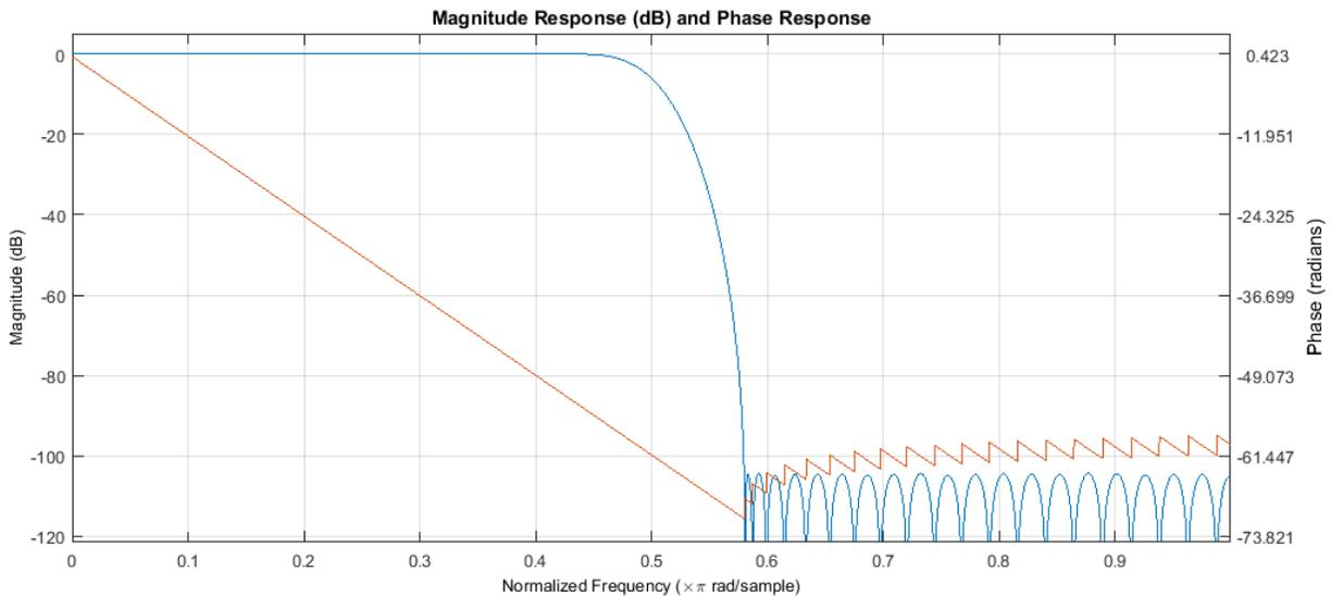
**Figure 2-4 Halfband Filter Frequency Response**
