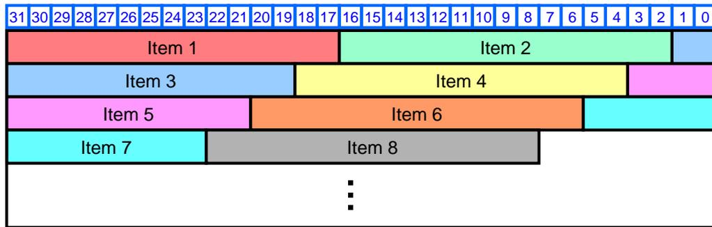
**Figure 3-6 Link Efficient Payload Organization**
