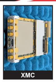
The SigStream<sup>™</sup> product family transforms a general purpose computer into a high speed signal acquisition/generation platform. The hardware incorporates a rich set of software programmable features that include selectable operating modes, external or timed event triggers, timestamped data samples, and flexible data formatting.
