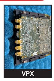
Four AC coupled 16-bit ADC channels
