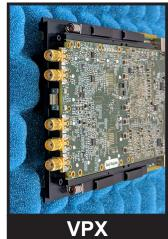
Two AC or DC coupled 16-bit ADC channels Two AC or DC coupled 16-bit DAC channels Internal or external sample clock (≤ 250 MHz) Phase locked frequency synthesizer Internal or external 10 MHz reference Selectable triggers (HW, SW, TOD) Continuous, snapshot, periodic operation ANSI/VITA 49 compliant data format Temperature and power supply monitors PCI Express (PCIe) x8 or x4 host bus High performance scatter-gather DMA Front and rear auxiliary connectors Demostration software (C) with source
